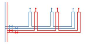
In the closed circular pipeline, a faultless installation in terms of hygiene is ensured as an optimum water exchange always takes place in the pipeline. Because the consumer is supplied from two sides, smaller pipe dimensions can be selected which also supports the water exchange.
