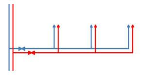
In drinking water distribution, T-piece distribution, series connection with U-shaped wall brackets and closed circular pipelines with U-shaped wall brackets are differentiated between. For reasons of hygiene, the "classic" T-piece distribution should only be used at consumption locations which are used regularly and daily. A minimum hygiene risk cannot be ruled out as stagnating water remains in the short supply lines to the consumers.
