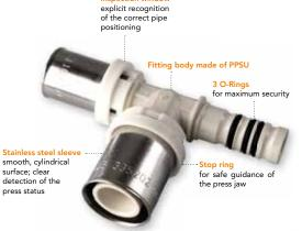
It is not necessary to use lubricants or other chemical substances during installation. Although PPSU can withstand a huge number of chemical agents, the contact to additional substances has to be avoided. Should this be necessary nevertheless, a clearance for the substance in question has to be obtained from MAINCOR
